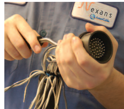
Service loops are completed at our 80,000 sq. ft. manufacturing facility in Houston, Texas. Bundles are inserted in hoses and fully potted (non-potted also available). Our highly experienced technicians add couplers/connectors as specified, then each loop is computer tested and packaged in weatherproof containers.
