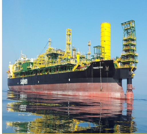
FPSO (Floating Production Storage and Offloading)
