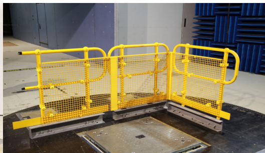
Wind Tunnel testing to determine C_{fig} value: Standard Metreage Assembly
